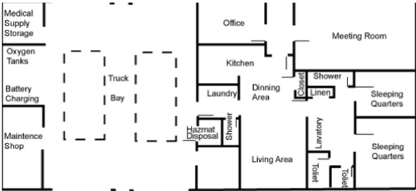
Figure 3. Example Floor Plan of a Two-Bay Building for a Rural EMS System
