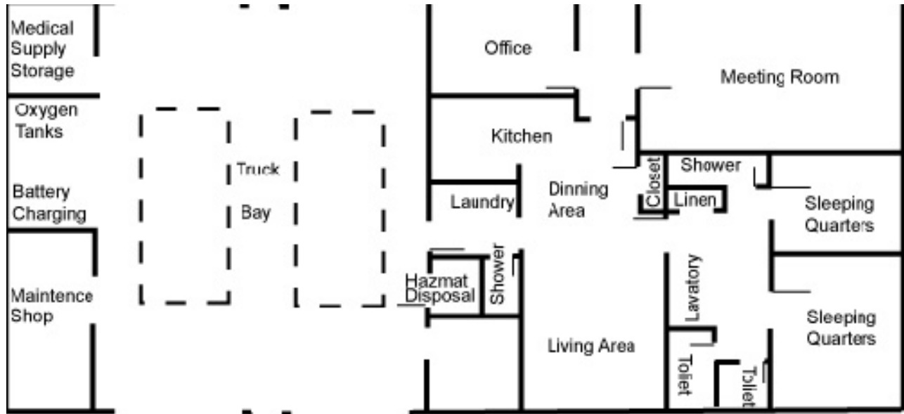
Figure 3. Example Floor Plan of a Two-Bay Building for an EMS System
